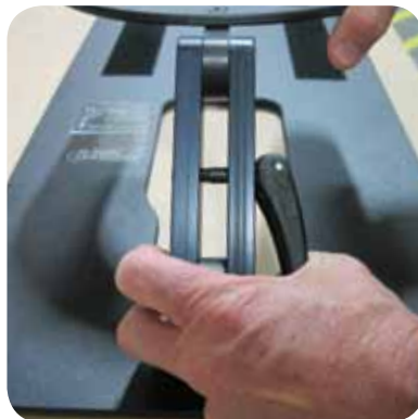
Step 4 - Force will increase as cam is near final position. Close cam to the final position
